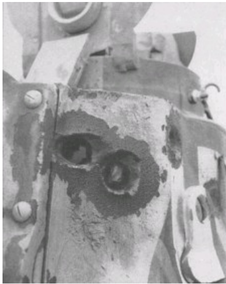
The thick turret of a Matilda holed in three places by a German anti-tank gun
