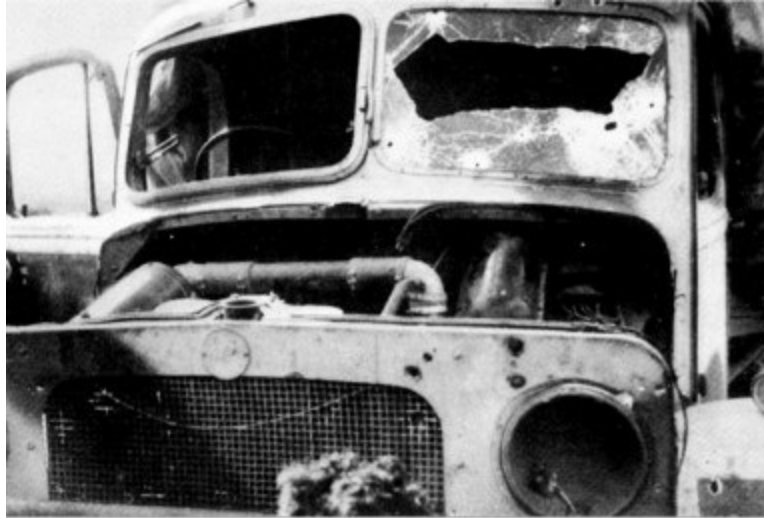
Driver's windscreen removed for visibility Driver's windscreen removed for visibility
